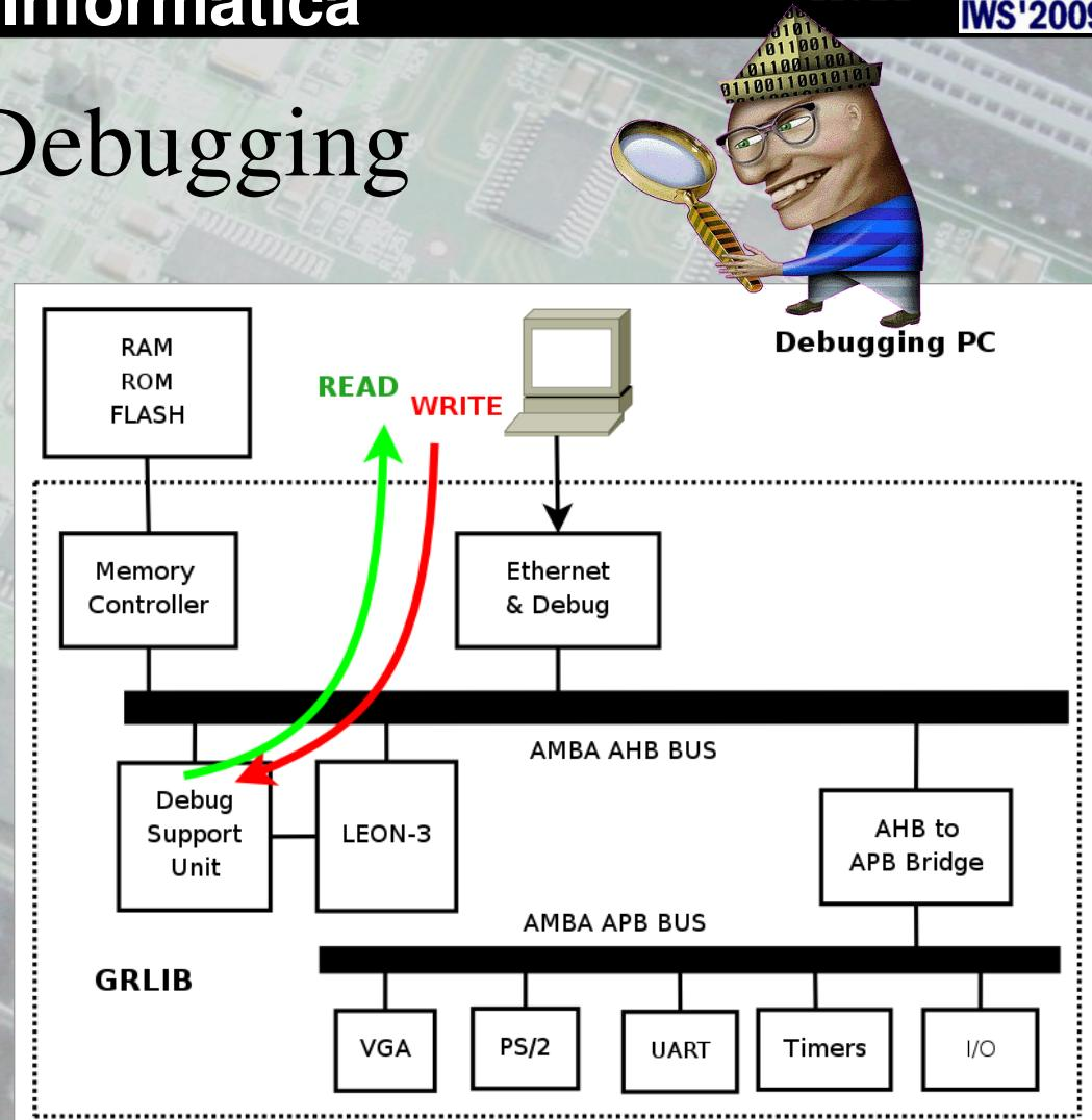
*Example: Debugging the LEON processor through Ethernet.*
